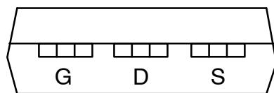
**Note:** Drain connected to metal part of mounting surface.
